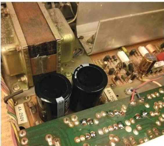
Showing the final power amplifier board with freshly replaced capacitors.
